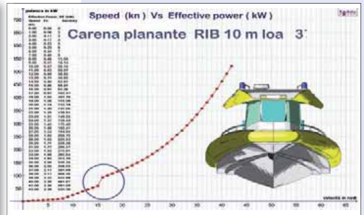
Fig. 2 - Curva tipica di resistenza monocarena planante / Typical resistance plot to a gliding monohull
