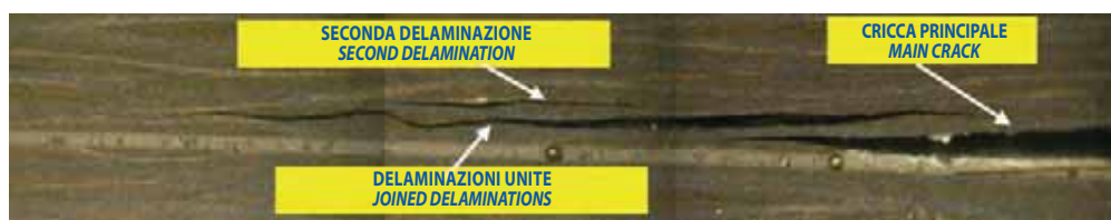
Fig. 8 - Delaminazione unite, MM = 0.15 / Joined delaminations, Mode Mixity = 0.15
