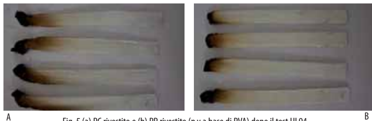
Fig. 5 (a) PC rivestito e (b) PP rivestito (p.v a base di PVA) dopo il test UL94 (a) Coated PC and (b) coated PP (PVA based coating) after UL94 test
