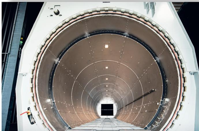
1 x 120° C class autoclave with an operating pressure of 4 bars (50 x 1.8 m)
